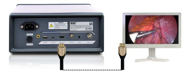
Connect the camera controller to a video monitor using the HDMI cable provided along with the unit.
