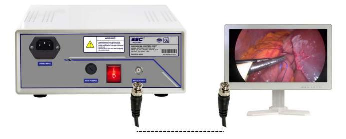
Connect the camera controller to a video monitor using the Video cable provided along with the unit.
